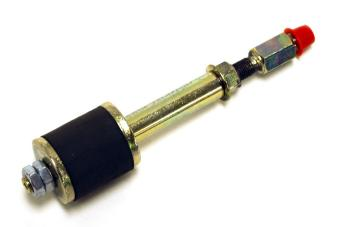
EST Group's Bolt Type Medium Pressure Test Plugs are designed for simple, reliable testing of pipe and tubing to 250 psig (17.2 bar), without the tube wall damage associated with other test plugs. That's because our Bolt Type plugs feature a neoprene seal — the only part of the plug that comes into contact with the tube ID. To use, simply install into the open end of the pipe or tube and tighten the large compression nut to expand the seal element. Then begin testing.
