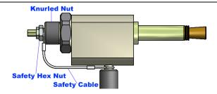
Failure to correctly seat and tighten hydraulic fittings will cause ram piston to lock in extended position after activation.
