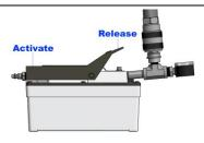
If plug does not "POP" and PsiG exceeds 7000 PsiG (483 BarG) on gage, STOP. Depress front of Hydraulic Pump pedal and Hydraulic Ram will retract. If the ring has not contacted the tube ID and plug can be removed from the tube on this first stroke you may have an UNDERSIZED PLUG. Otherwise tighten knurled nut and depress pump pedal. If plug does not "POP", on second stroke an UNDERSIZED PLUG has been installed, stop and contact EST Customer Service, or your local representative for assistance.
