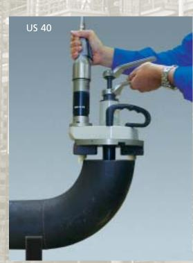
Using it will eliminate the harsh work of manual beveling with its costly time and imperfection.
