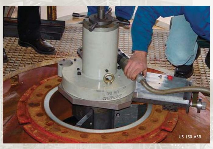
The flange facing attachment has been designed to be quickly adapted on any standard pipe beveling machine of our range, to further multiply its use by also allowing it to resurface all the different flanges welded on pipes, directly onsite.
