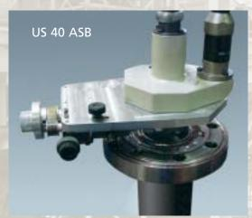
It may be used by clamping the machine directly inside the pipe, or if an extreme squareness and centering is required, the spider shaped elbow mandrel kit will be necessary.
