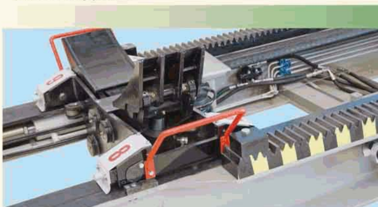
Hydraulically controlled bundle supports
