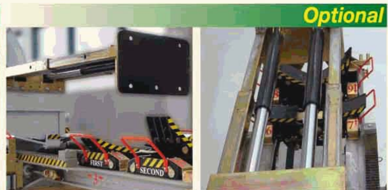
Hydraulic telescopic extended arm for bundle insertion
