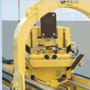
Circular rocker arm for lifting
