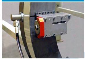
100 mm stroke carriages or two ovalization tracking carriages are necessary. Depending on the application, A wide range of cutting or beveling tool-bits are available, allowing to perform the majority of the required machining applications.
