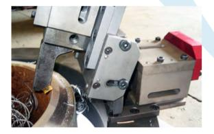
The counterboring carriage allows to perform an ID bevel to get a regular land.
