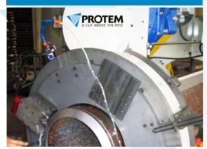
In order to increase the lifetime of the inserts and to reduce the noise level during the machining works, a lubrication device shall be used: This lubrication device is made up of a cutting fluid tank, cov ered by a chip container and a pump for circulating the cutting fluid . A flexible piping kit for aiming the fluid at the cutting point is also supplied together with a tank support plate. This option is activated through a push button.
