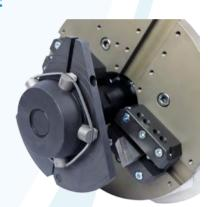
Step 2: Machine clamping: No adjustments needed. The device is self-centering because of the concentric jaws.
