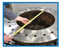
Set machine onto flange using setup fingers. Lightly tighten leveling feet in the flange.
