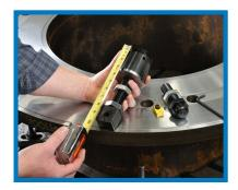
Extend feet into flange. Indicate, level and tighten leveling feet and stationary feet.
