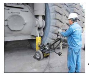
Enerpac POW'R-RISER<sup>®</sup> used in mining operations to lift heavy equipment.
