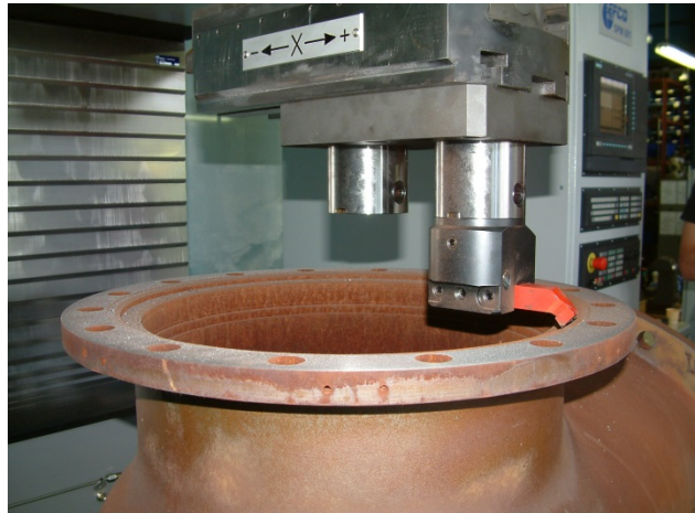
Face turning of flanges
